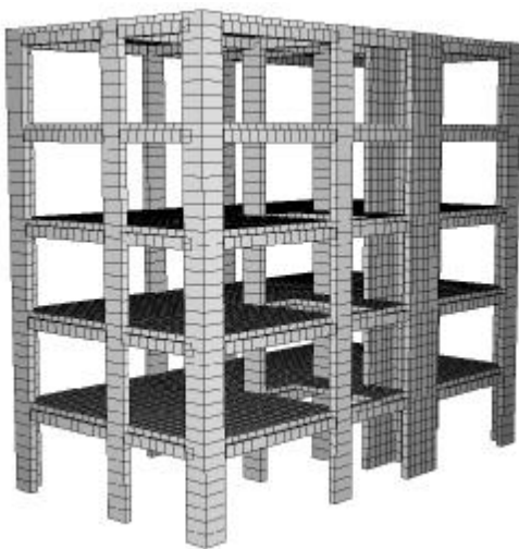
Fig. 2: Finite element model of the structure
