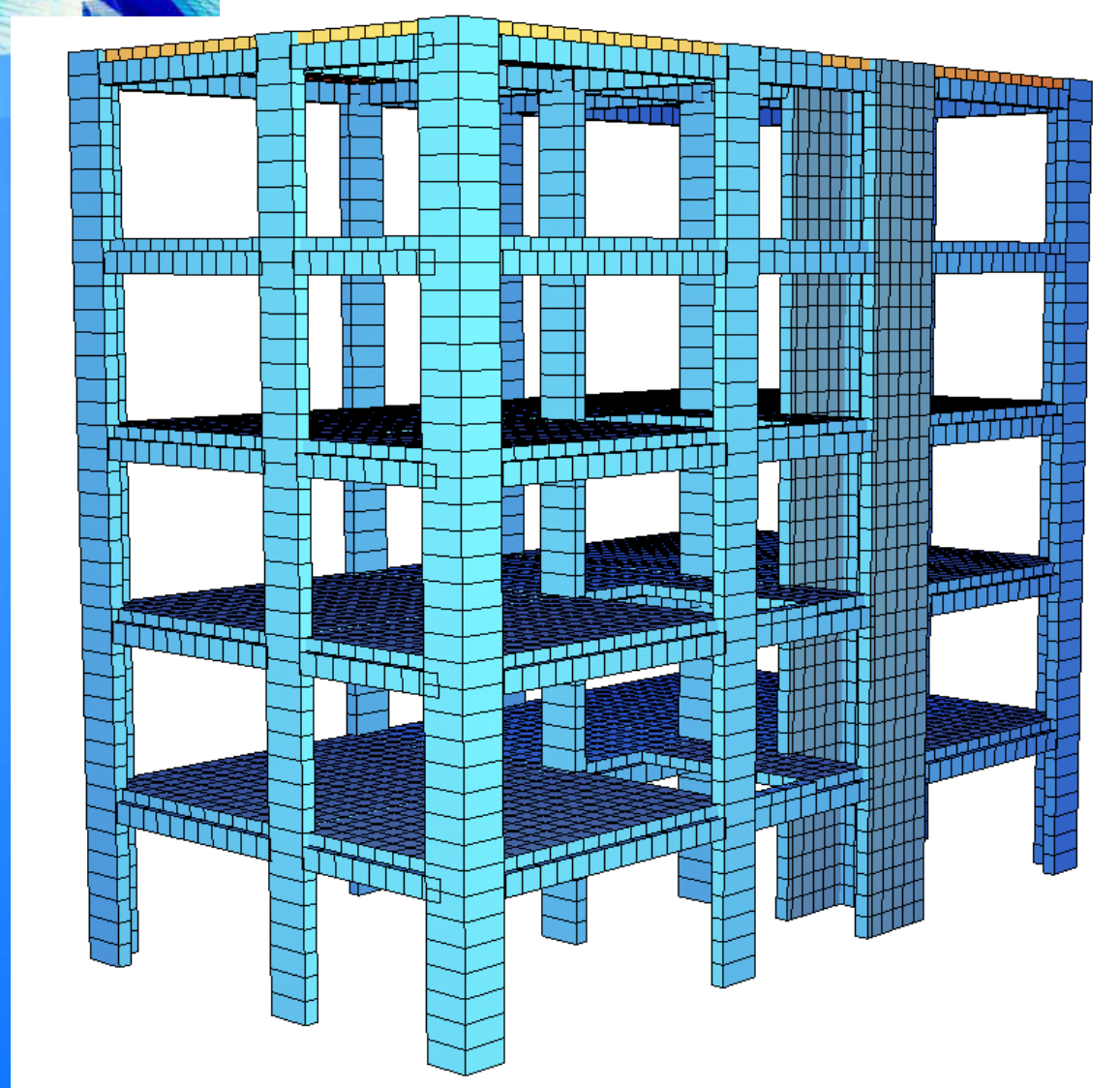
Finite element model of the structure
